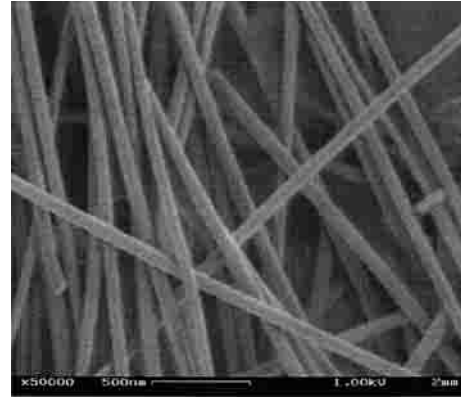
Fig. 1. Electrodeposited Co nanowires observed with high performance scanning electron microscopy after dissolution of the polycarbonate membrane in dichloromethane. The average wire diameter is 90 nm.
